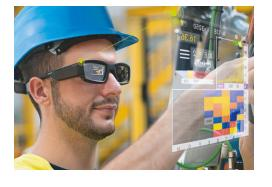
EM5000 thickness gauge can be supplemented with wearable smart glasses upon your request. Wearable smart glasses allow using EM5000 EMA thickness gauge in hard-to-reach places, where display readouts are impossible or difficult. In this case the readouts are displayed on the lenses of the smart glasses and the operator can always see them.
