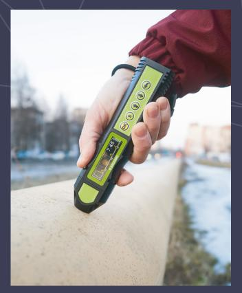
Designed for thickness measurement on steel pipes wall, flat steel, steel flat bars or steel sheets, aluminum and other metals, with a operating gap of up to 4 mm between the sensor and metal.
