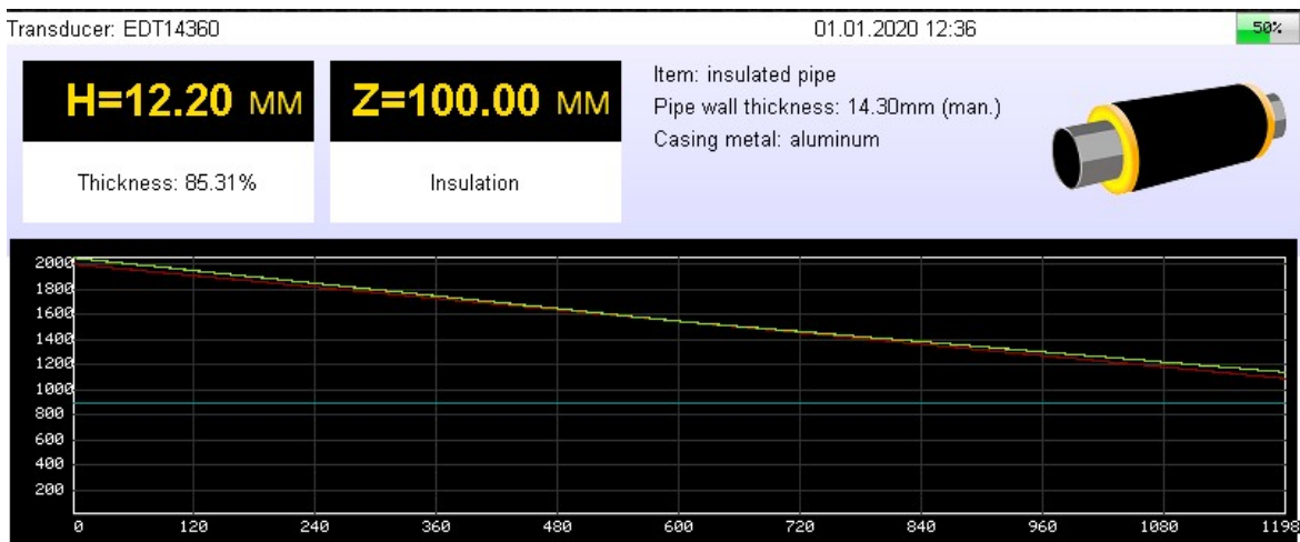
Figure 46. Unavailable point of crossing the threshold on A-scan
