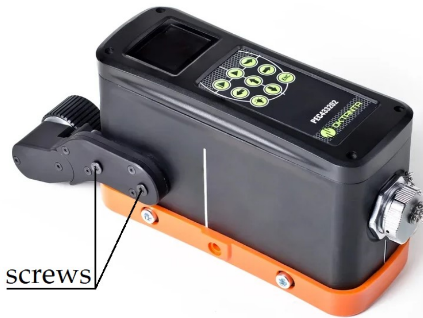
Figure 59. Encoder layout on the sensor.
