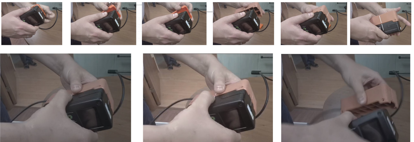
Figure 42. The replacement of plastic and rubber protectors.
