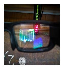
EM2210 mini thickness gauge can be supplemented with wearable smart glasses upon your requst. Wearable smart glasses allow using EM2210 EMA thickness gauge in hard-to-reach places, where display readouts are impossible or difficult. In this case the readouts are displayed on the lenses of the smart glasses and the operator can always see them.
