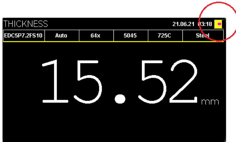
Battery charge indicator
